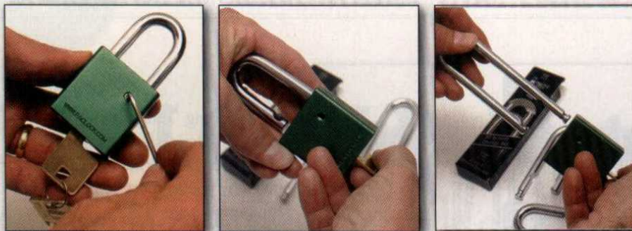
Left: Remove Hex Shackle Retaining Screw; Center: Release Shackle; Right: Install New Shackle
