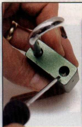
Left: Remove Cylinder Retaining Screw; Center: Access to Actuator; Right: Remove Actuator
